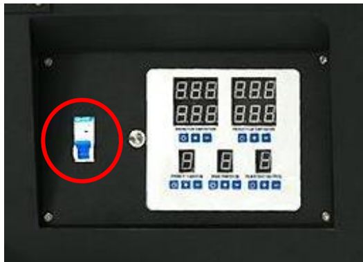
C. Main Power Switch:
